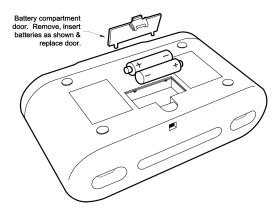
Flip the unit upside down, remove the battery cover, and install two **AA batteries** in the battery compartment. Follow the polarity markings inside the battery compartment. Replace the cover.
